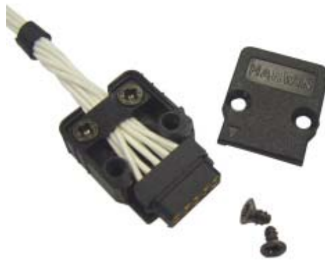
Figure 4: Cable assembly with cover
